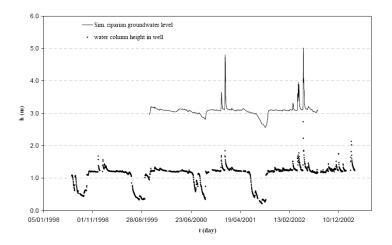
Figure 7. Comparison of the temporal dynamics between the point water column observed in a well located in the riparian zone near the Fuirosos stream channel and the riparian groundwater table simulated by the model SD4-R.
