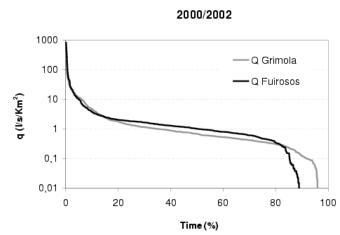
Figure 2. Specific daily stream discharge ordered from the highest to the lowest for the Fuirosos catchment and the Grimola subcatchment for the period from 18/09/2000 to 22/08/2002.
