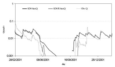
Figure 5. Influence of the riparian zone on the transition period simulation. The thick black line represents the simulated discharge obtained with the SD4 model, which does not include the riparian tank; the thick grey line represents the simulated discharge by the SD4-R model and the thin grey line represents the observed discharge.
